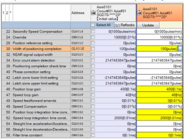
(2) Added the function to reflect the "Current value" of the Auto-update Parameters in the "Initial value".
