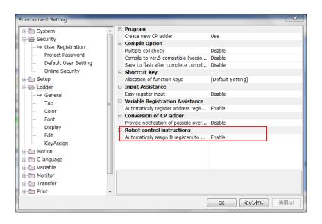
(4) In the property screen of each ladder program, added the setting of the First Address of the D register to automatically arrange the D register variable of the unused area of (2).
