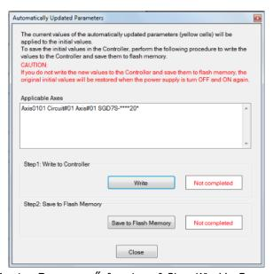
(4) When the "Update Auto Reflection Parameters" function of SigmaWin+Ver.7 parameter edit screen was operated, improved so that the set value converted using the machine specifications of the fixed parameter of the controller was reflected in the positioning completion width at "OLxx1 E" of the setting parameter.
