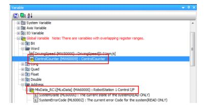
(4) When it expanded "global variable" in the state of the previous section, the variable list of duplicate states were made to be displayed. In addition, duplicate user registration variables could be deleted all together on this screen.
