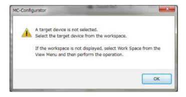
(2) The prefix of the name that displayed in the target device selection list on the workspace screen was displayed as "Axis" even on the I / O device.
