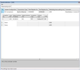
(3) When there were duplicate user registration variables for the registers that set in the detailed definition of SVK, a warning was made to be displayed in the variable window.
