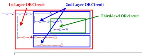
1 st level OR circuit: OR circuit branched from Lang's busbar 2nd layer OR circuit: OR circuit branched from within the 1 st level OR circuit 3rd level OR circuit: OR circuit branched from within the 2nd level OR circuit
