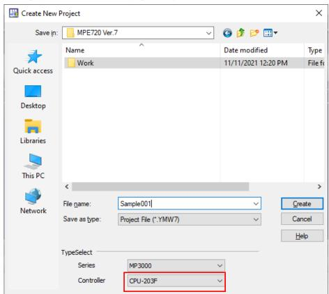
2) It can be connected to the CPU-203F controller for engineering.
