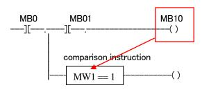
MB000010 (MW00001) is referred in the comparison instruction of the next OR circuit.
