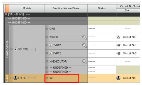
2) You can set the relay connection via IoT unit in the communications setting. You can edit the data sharing settings by using MPE720 on the PC installed YASKAWA Cockpit.
