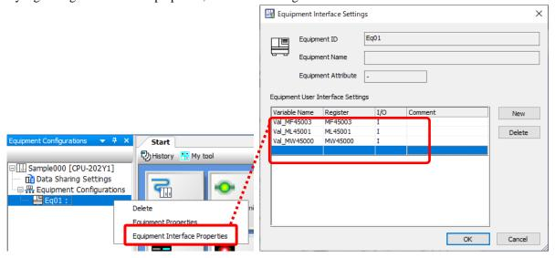
4) The data handled by the CPU unit of YRM-7 can be shared with the IoT unit. Thereby, the data can be collected from YASKAWA Cockpit and fed back to.
