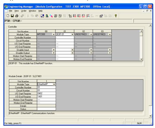
The 263IF-01 module(EtherNet/IP) has the function of EtherNet/IP that mounts standard (EN50170, IEC 61158)CIP (Common Industrial Protocol) where results exist in DeviceNet in the TCP/IP protocol of standard Ethernet. The EtherNet/IP function can handle the I/O message and the Explicit message.
