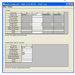
262IF-01 is a communication interface to connect the MP series Machine Controller with FL-net (OPCN-2).
